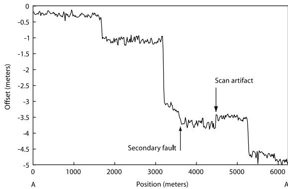
Fig. 5. Profile AA' from Fig. 2. Secondary fault with slip amplitude as low as 20 cm is detected and its location is indicated by a black arrow on Fig. 2. At around the same amplitude a scan artifact is also detected and is indicated by a white arrow on Fig. 2. The standard deviation of the measurements is 7 cm.
