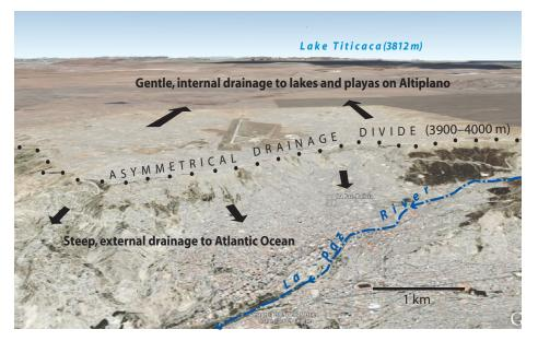
Figure 14. GoogleEarth<sup>™</sup> image looking NW over the city of La Paz, Bolivia, onto the Altiplano toward Lake Titicaca. Headward erosion of the La Paz River drainage has created an asymmetrical drainage divide with steep SW slopes draining to the Atlantic Ocean and gentle NW slopes that lie within 200 m of the level of Lake Titicaca.
