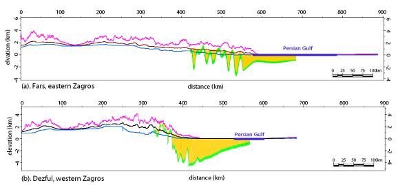
A long N-S topographic cross section across the Zagros fold thrust belt with maximum (pink), mean(black) and minimum (blue) elevations within a 100-km-wide swath extracted from the SRTM 90 m digital elevation model. The Asmari formation (green unit) is extracted from published cross sections and boreholes by National Iranian Oil Company. The Neogene foreland deposits are shown in orange.
